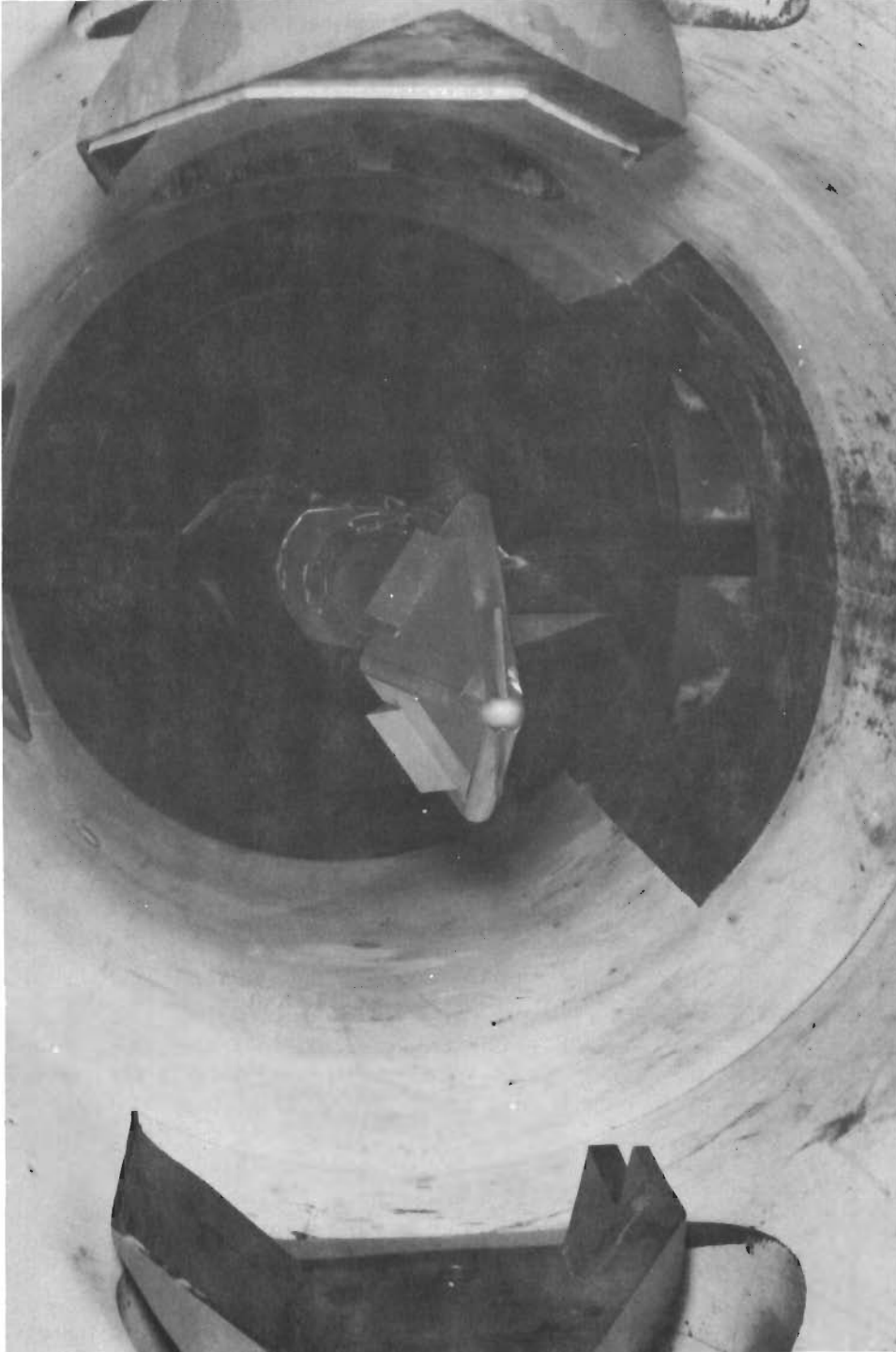
Fig. 2a Photograph of Model, with Canards and Upper (Dihedral) Flaps Deflected, Installed in the AEDC 50-inch Mach 8 Tunnel
