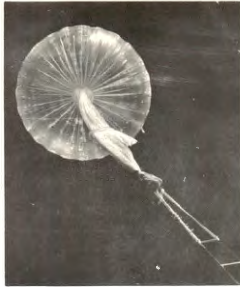
Figure 4. Start of Gas Transfer - 42,000 Ft
