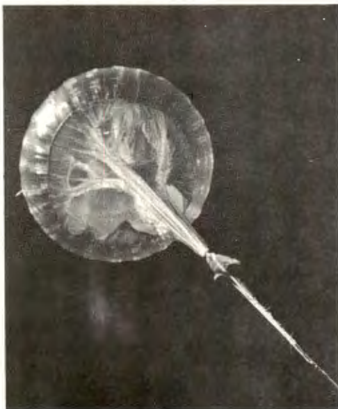
Figure 5. Main Balloon Supporting One-Third of Load
