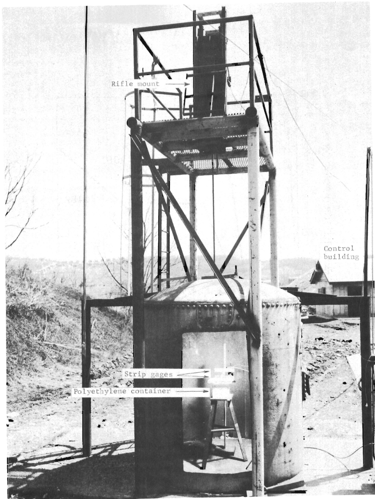
Figure 3. - Facility used to conduct experiments on shock sensitivity of solid oxygen-liquid hydrogen mixtures.
