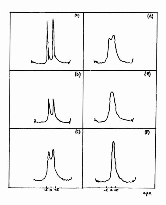
'H Spectra of Phenyldimethylaminochlorobornie at Several Temperatures (4) 23°, (b) 93°, (c) 103°, (d) 109°, (e) 118°, (f) 137°.
