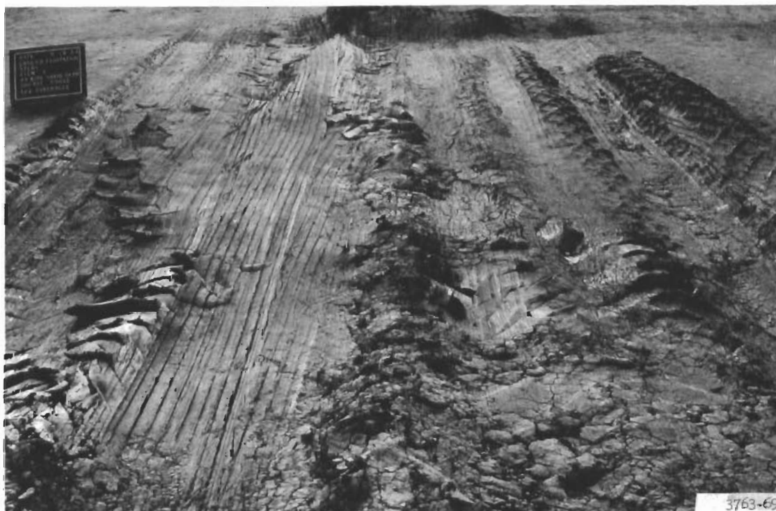
Figure 15. Lane 3, item 3, at 122 coverages (62 postfailure coverages)
