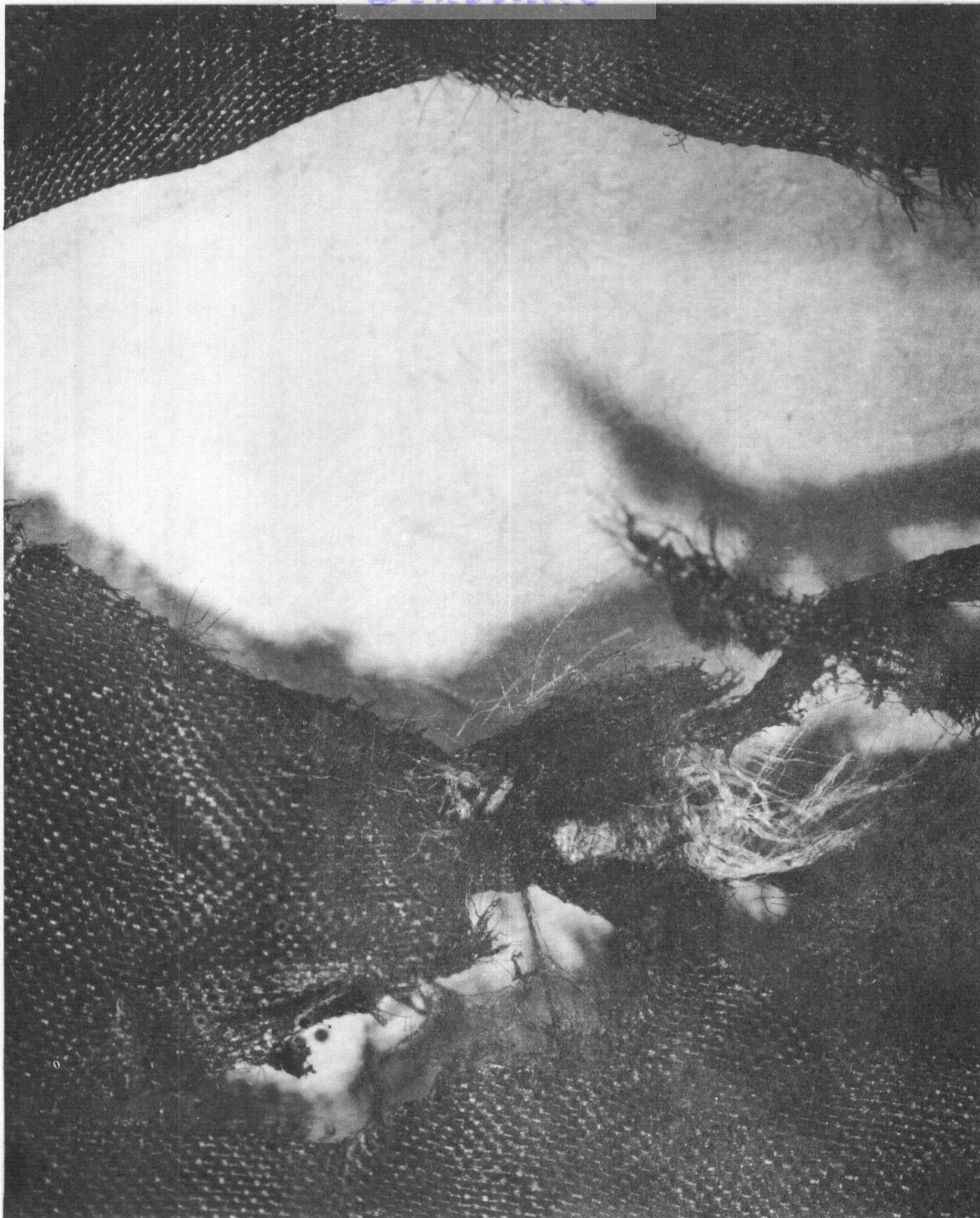
Figure 108. Damaged Fabric Due to Rubbing.
