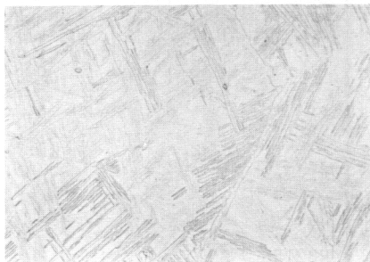
e. Medium Acicular Alpha, Solution Heat Treated
