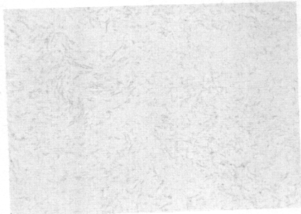
a. Fine Equiaxed Alpha, Stabilized
