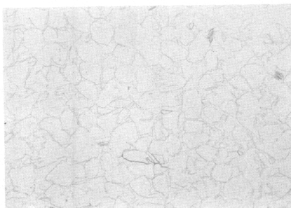
h. Coarse Equiaxed Alpha, Stabilized
