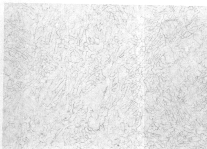
h. Coarse Equiaxed Alpha, Stabilized
