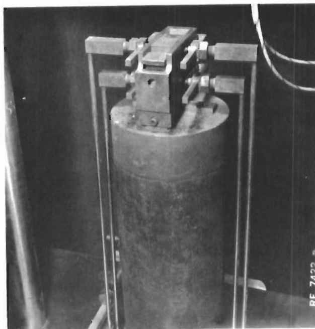
FIGURE 32- COMPRESSIVE TEST ARRANGEMENT
