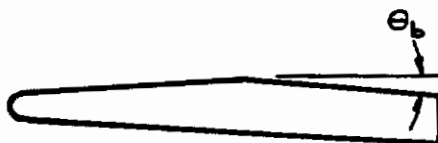
FIGURE 40. Method for Determination of Geometrical Parameters for Configurations Having Unsymmetrical Boat-tailing
