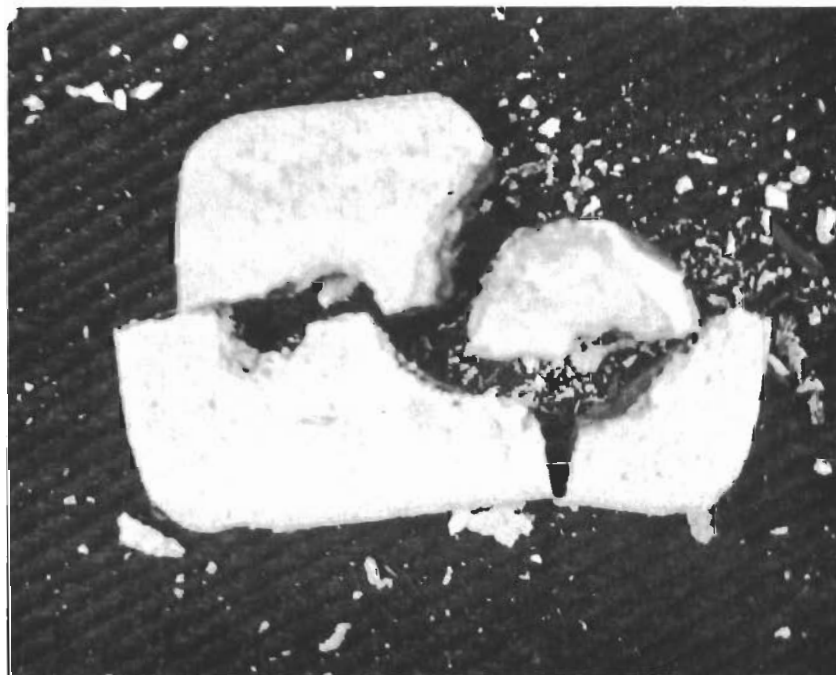
a. Si Coated, Cyclic Life 9.5 Hours at 2500 F
