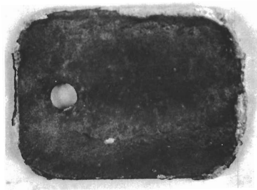
b. Cr-50Ti Coated Tantalum, Failed in 2 Minutes
