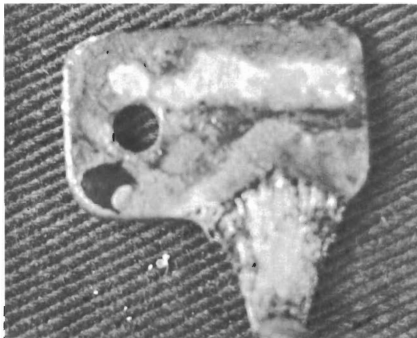
e. Exposed at 2500 F, Average Cyclic Life Greater Than 20 Hours
