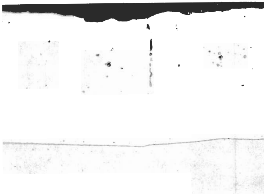
b. As Coated in Two Cycles, 4 Hours and 12 Hours, 3.7 Mil
