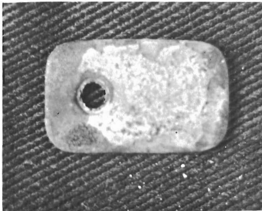
c. Exposed at 1800 F, Cyclic Life Greater Than 100 Hours
