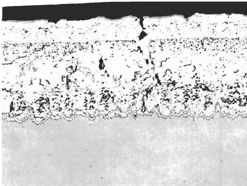
b. Calculated Si-79B Coating Applied to Tantalum by Boronizing for 4 Hours and Siliconizing for 12 Hours at 2200 F, 7.2 Mil
