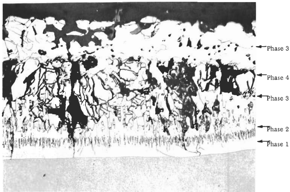
b. Si-26Mn Coated Tantalum as Coated at 2200 F
