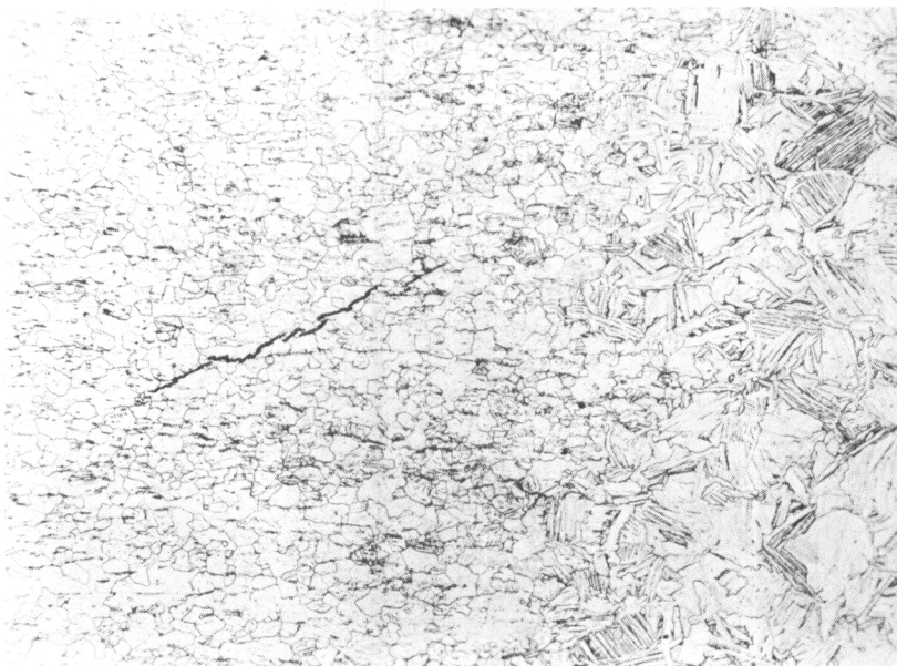
FIGURE 18. CRACK IN UN- AFFECTED BASE METAL JUST OUTSIDE HEAT-AFFECTED ZONE OF WELD IN TITANIUM - 0.30 PER CENT OXYGEN-ALLOY SHEET
