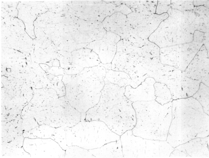
FIGURE 8. TYPICAL ANNEALED STRUCTURE OF TITANIUM SHEET USED IN THIS INVESTIGATION EXCEPT THOSE CONTAINING 0.28 PER CENT OR MORE CARBON.
