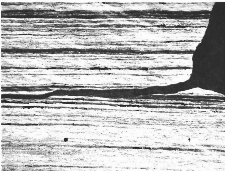
Figure 31. Typical Precrack-Charpy-Impact Fracture Surfaces in Transverse Specimens with Two Orientations of Notch, 18% Nickel Maraging Steel, Heat 13371
