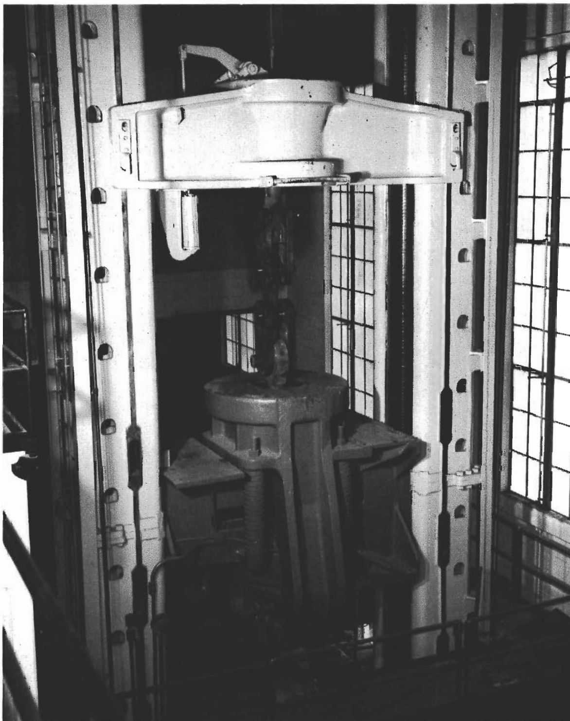
Figure 129. Four-Million lb Tensile-Testing Machine with Test Specimen in Place
