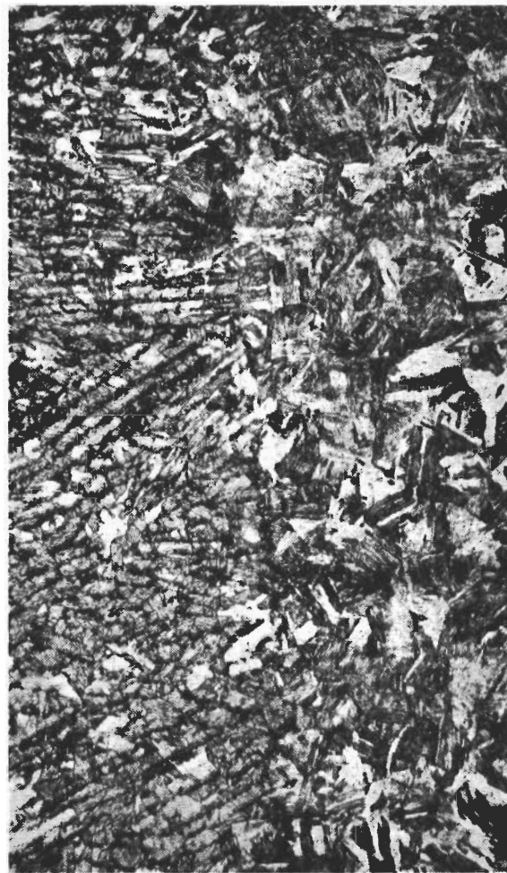
Marbles Etch Magnification: 250X WM HAZ
