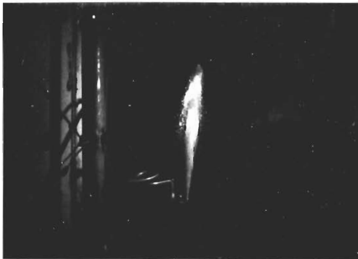
A. OVERALL VIEW OF RP-1 SPRAY FROM 1-HOLE INJECTOR — 70 MILLISECONDS AFTER START OF INJECTION, 100-110 PSI INJECTION PRESSURE.
