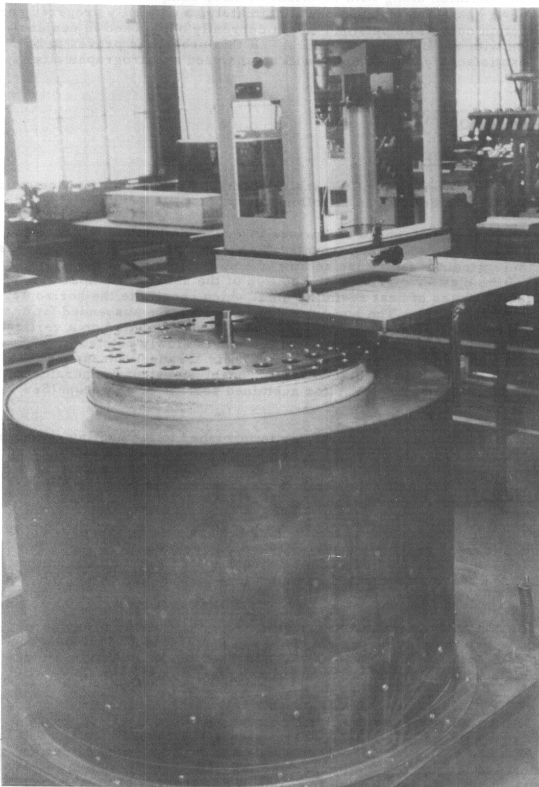
Fig. 4 View of assembled scaling furnace showing rotating top and balance.
