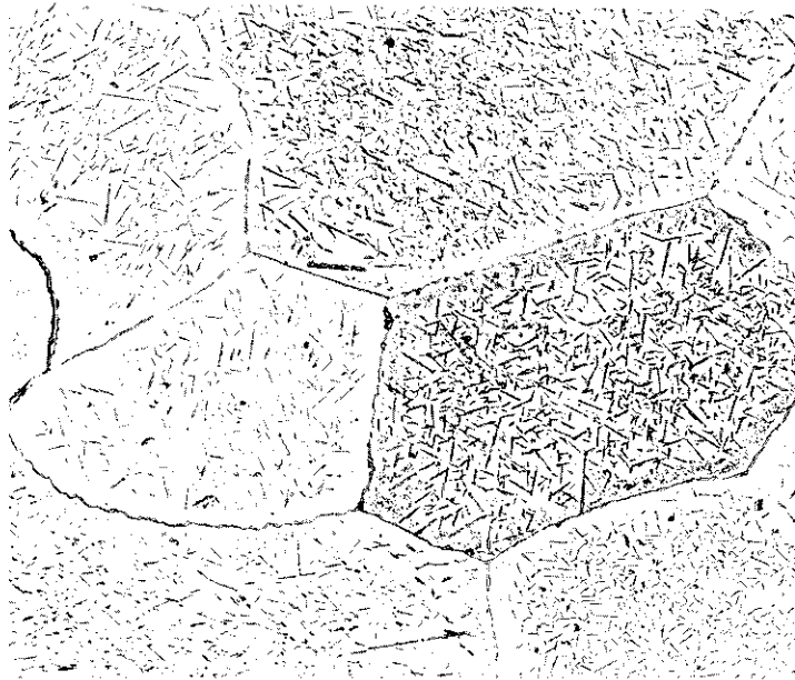
Nb-0.30 w/o C. As cast. 100x Nb 2 C precipitate in niobium solid solution.
