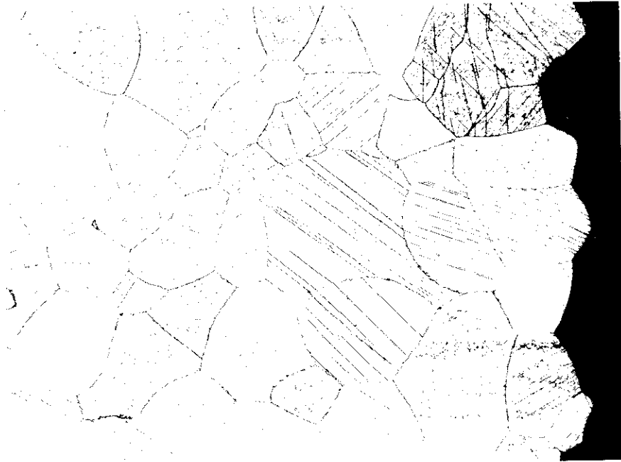
Fig.33—Deformation twins in Nb-20Ti alloy (NC-195). Annealed 1 hour at 1600 C prior to testing at -196 C. 100X
