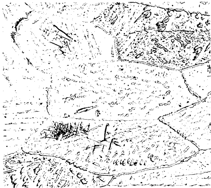
Nb-0.75 w/o C. As cast. 100x Nb 2 C precipitate in niobium solid solution.
