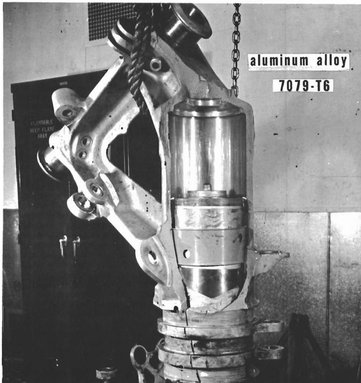
Figure 8. Stress Corrosion Cracking Landing Gear Cylinder
