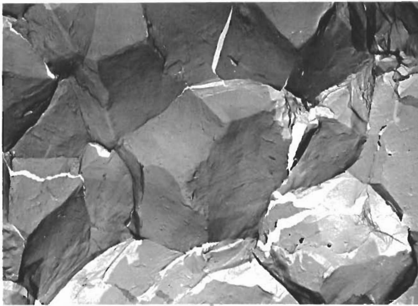
(c) Hydrogen Embrittlement Fracture AISI 4340 M (220-240 ksi UTS) 7000 x
