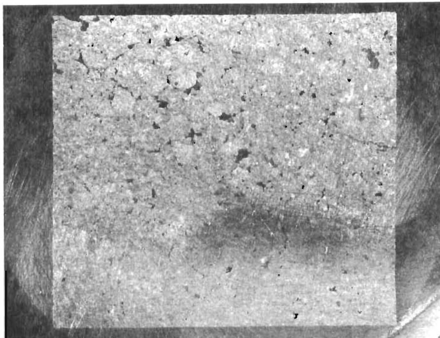
Figure 9. Graphite Specimen Surface After Grinding on 500-Grit Diamond Wheel, 7 X.
