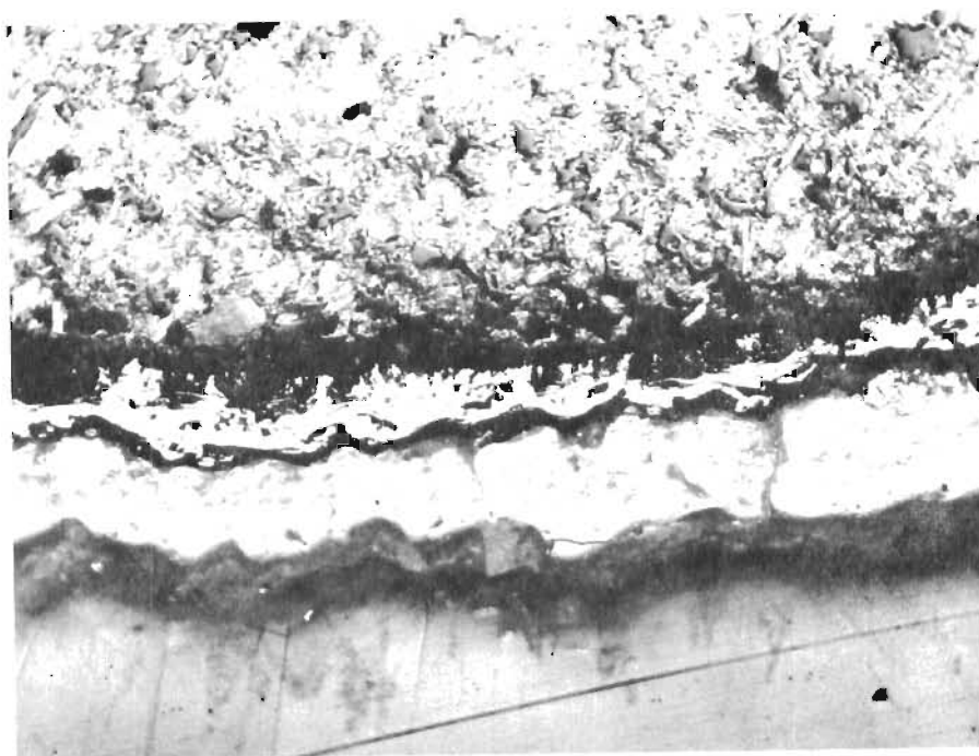
Figure 16. Relief-Polished Ceramic Coating on Graphite Substrate, Coating in Focus, 100 X.
