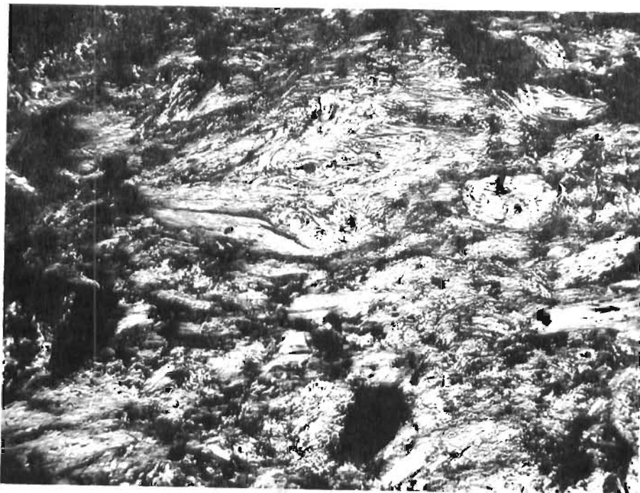
Figure 36. ZTE Graphite Photographed on High Resolution Plate, Developed in D-19, 100 X.
