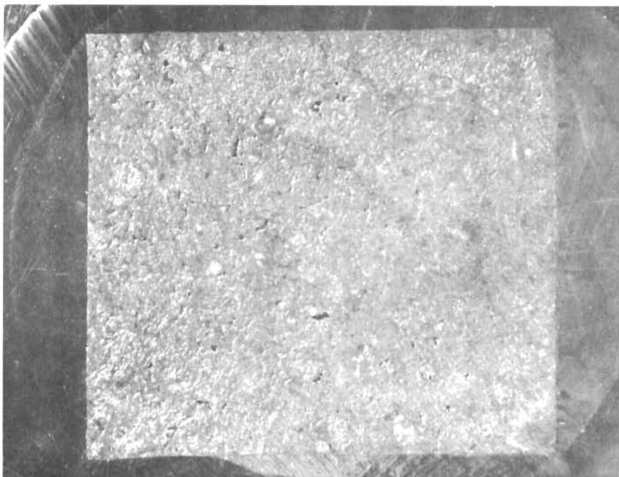
Figure 10. Graphite Specimen Surface After Polishing With 600-Grit Silicon Carbide Abrasive, 7 X.
