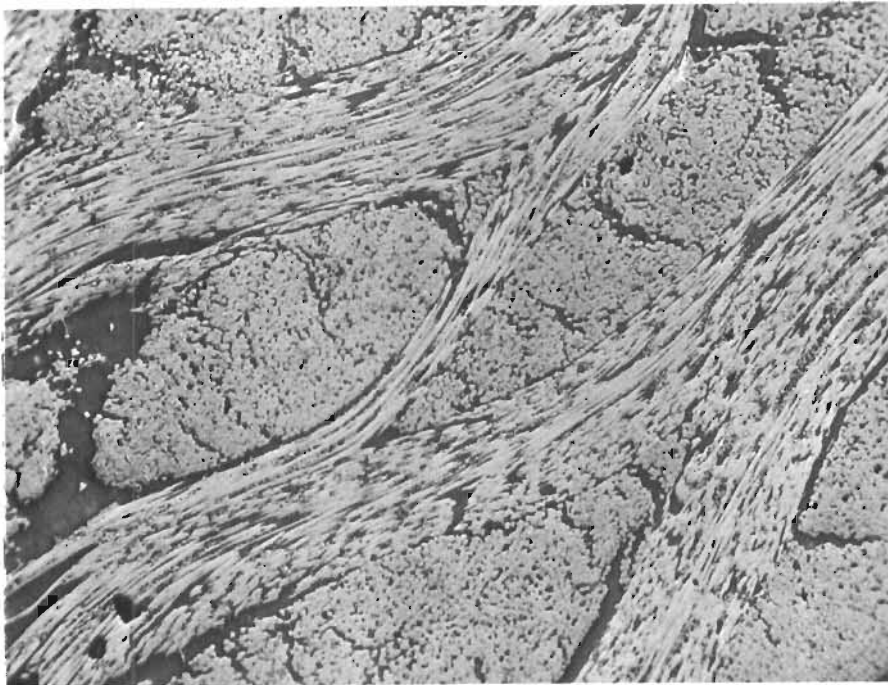
Figure 29. Graphite Cloth Using Bright-Field Illumination, 100 X.
