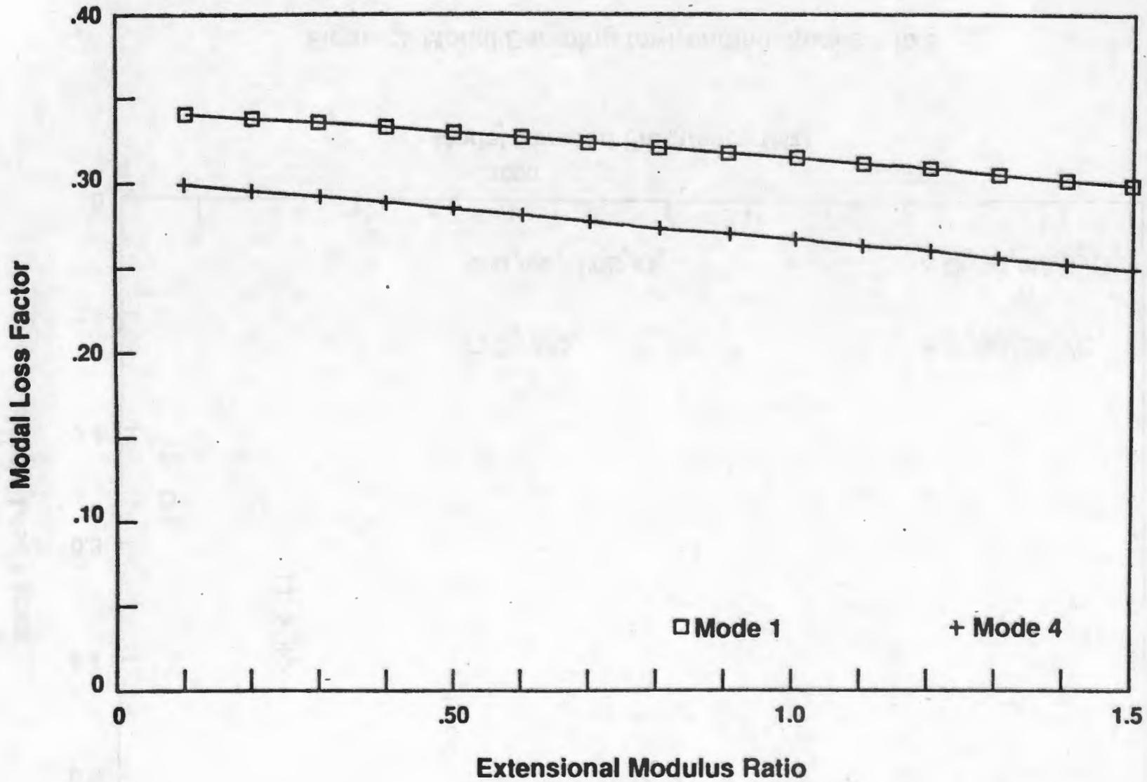
Figure 5 Modal Damping vs the Modulus of the Compliant Layer
