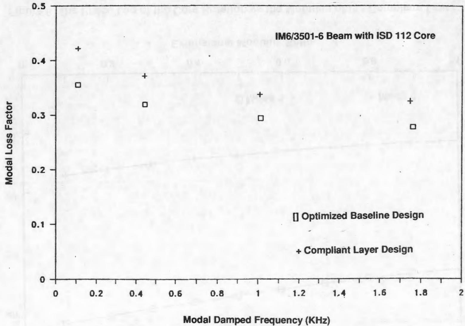
Figure 7 Modal Damping for Optimized Designs
