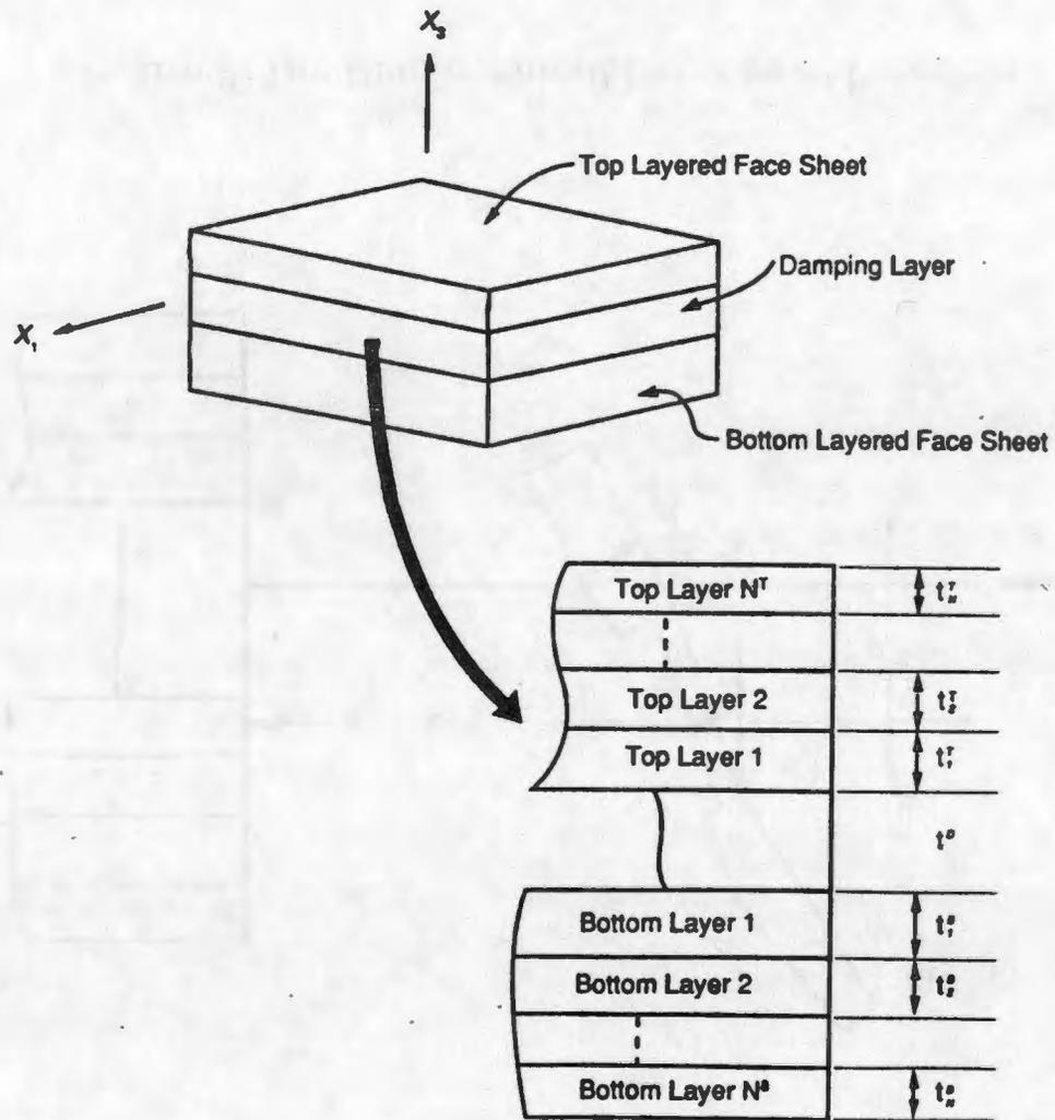
Figure 1 Damped Sandwich Beam
