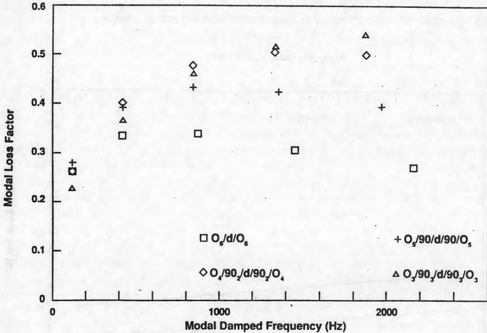
Figure 3 Modal Damping for Bending Modes 1 to 5
