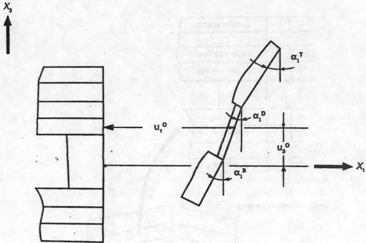
Figure 2 The Displacement Degrees of Freedom
