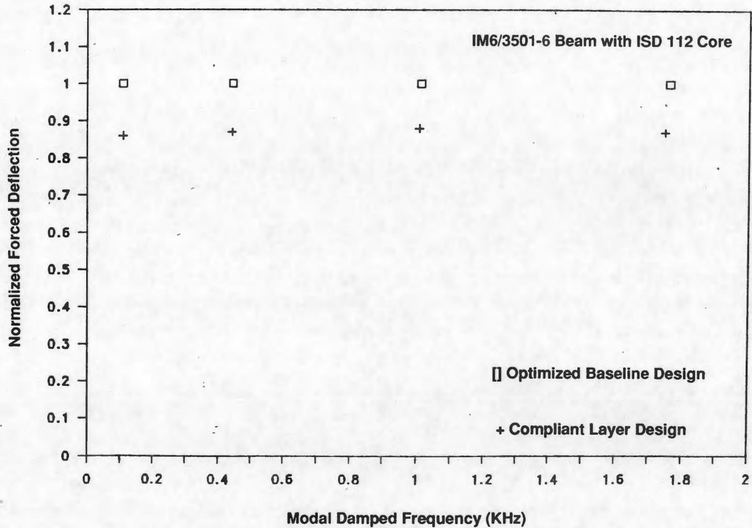
**Figure 8 Normalized Forced Deflection for Optimized Designs**
