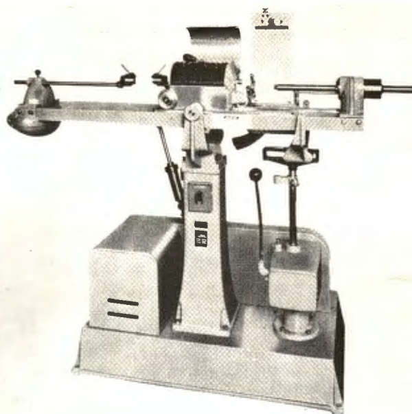
Figure 1. The Scott Inclined Plane Testing Machine for Constant Rate of Loading
