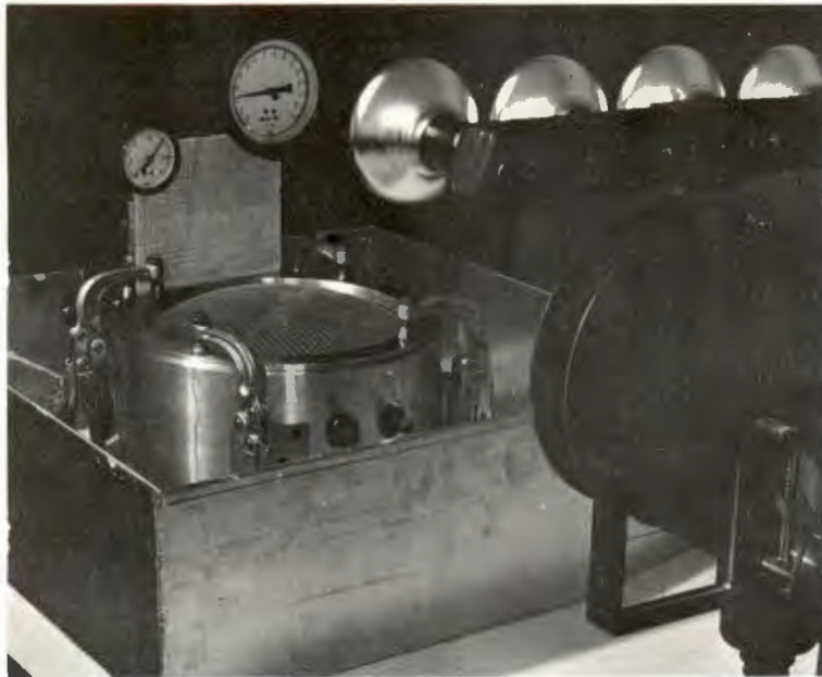
Figure 7. Photograph of Biaxial Equipment Testing a Scrim-Reinforced Balloon Material
