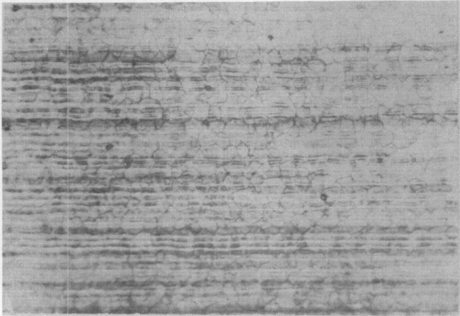
Neg. No. 33662 250x Etchant: Phospho Picral Alloy No. 71587 a.) Mg-5Al
