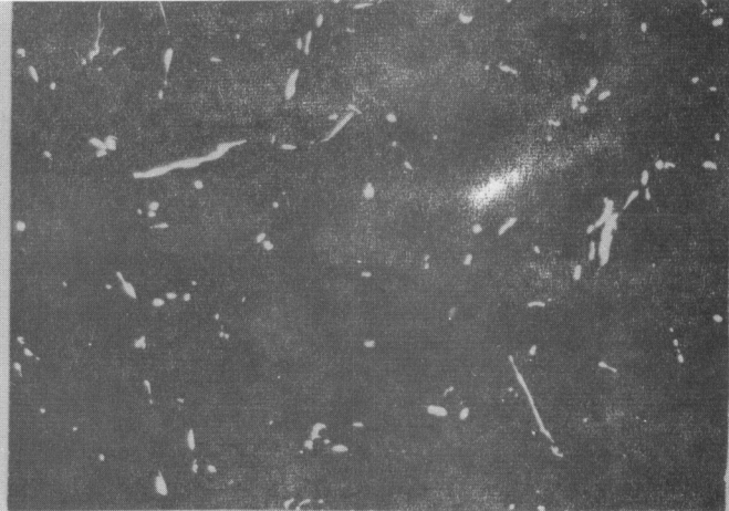
Neg. 31401 100X Alloy No. 71588 Etchant: Phospho Picral
