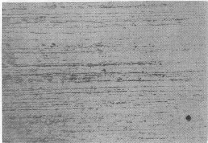
Neg. No. 33666 250x Etchant: Phospho Picral Alloy No. 71603 d.) Mg-5Al-1Ba
