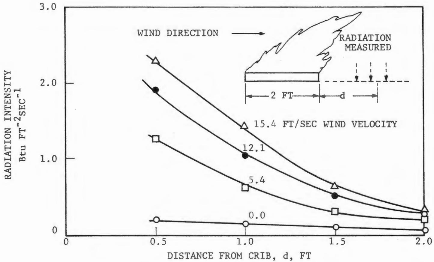
Fig. 5 EFFECT OF WIND ON RADIATION
