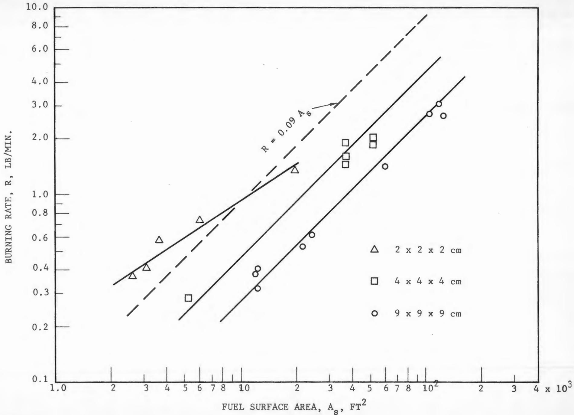
FIG. 3 BURNING RATES OF UNORDERED CRIBS AS A FUNCTION OF FUEL SURFACE AREA
