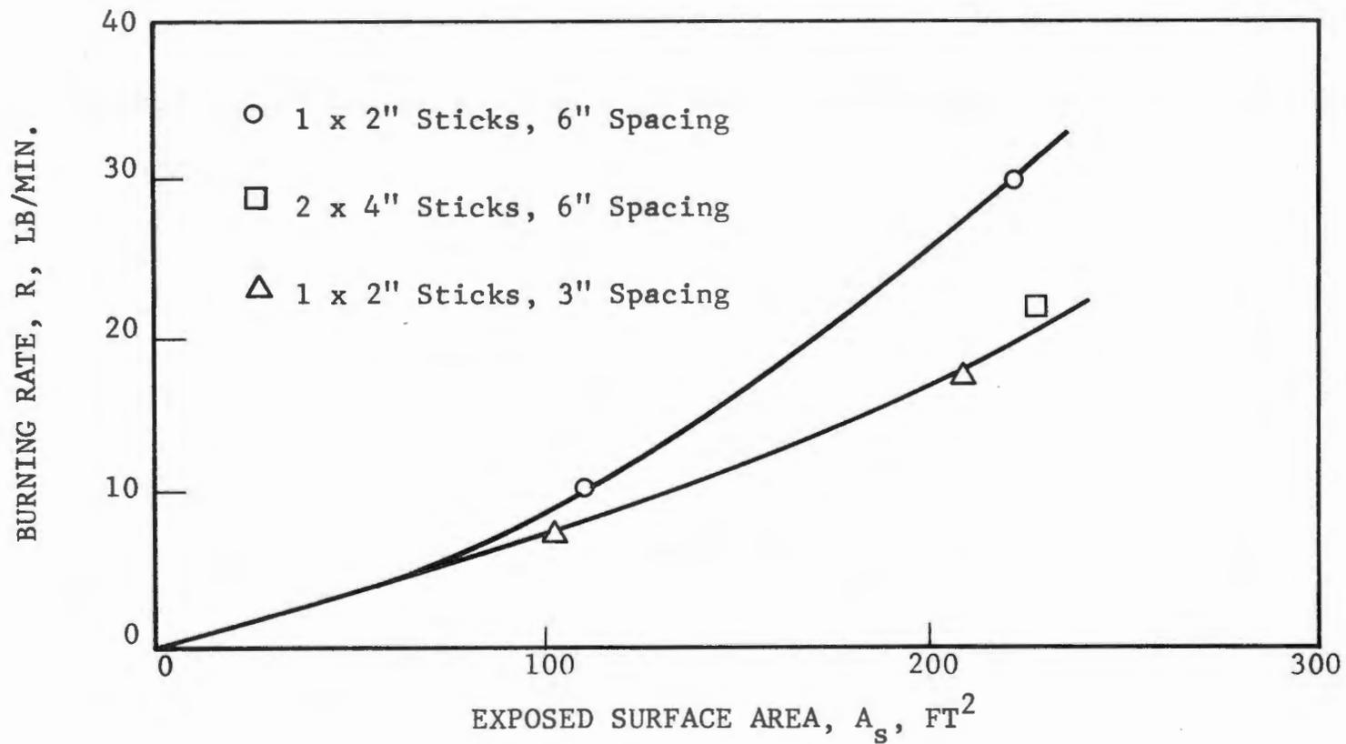
Fig. 2. EFFECT OF WOOD SURFACE AREA ON BURNING RATE OF 6 x 6 FT CRIBS
