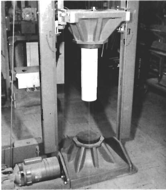
Figure 5 — Mounting of Attenuator to Varipulse Shock Machine.
